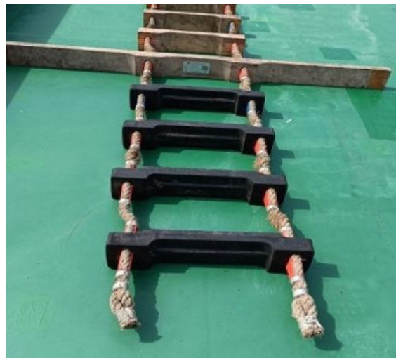
Starboard Side Pilot Ladder (Bottom Section)
