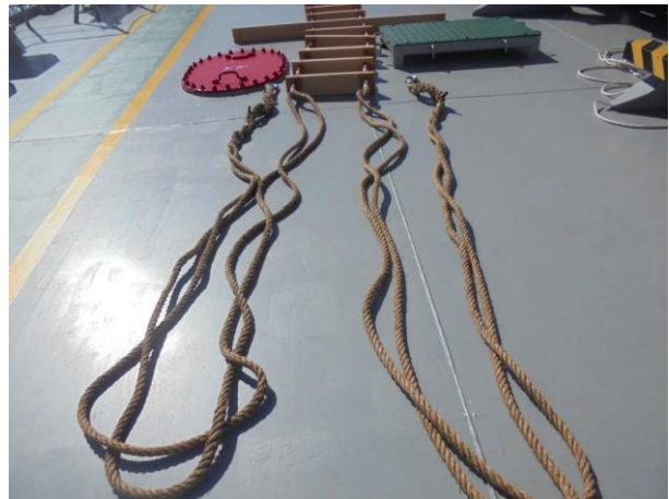
Starboard Side Pilot Ladder (Top Section)
