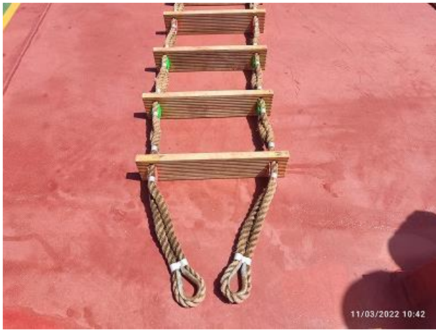
Port Side Pilot Ladder (Top Section)
