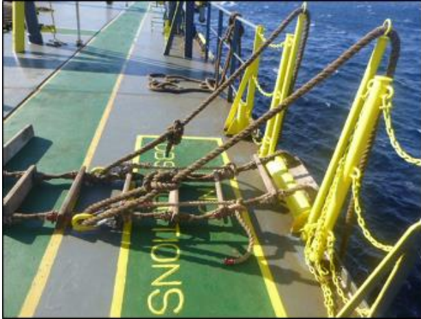
Securing strongpoints on deck for ladders and manropes
