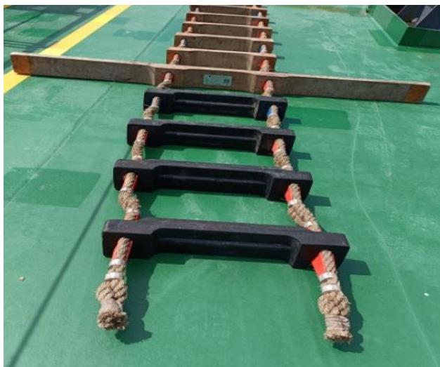
Port Side Pilot Ladder (Bottom Section)
