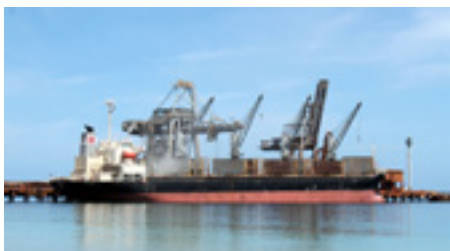
Bulk carrier MV Ken Mei unloading white clinker at the Kwinana Bulk Terminal for Cockburn Cement
