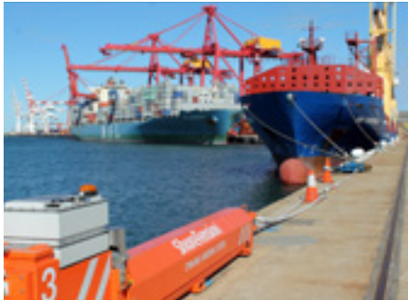
The ShoreTension hydraulic mooring system is deployed to increase safety and stability for ships in the Inner Harbour when stormy weather is forecast.
