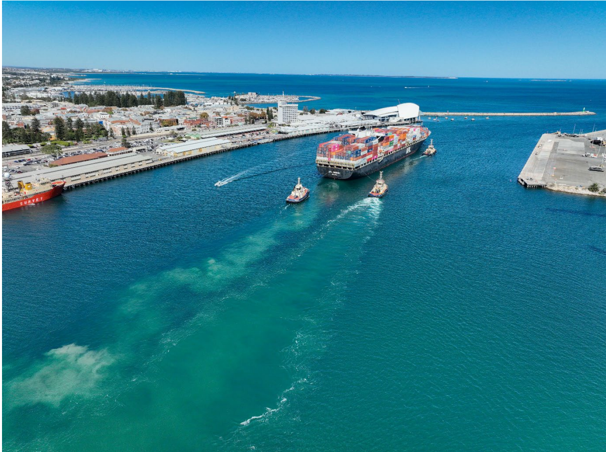
Figure 4: Drone aerial image from Zone 1 on 16/04/2024 showing a visible sediment plume created by a ship exiting the Inner Harbour.
